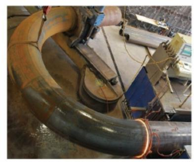
Most flexible induction pipe bending machines on the market. Most economic to run with patented technology. Simple to operate with PLC operation. Quickest tool set—up and cycle time. The most affordable induction forming solution when compared to other machines. The entire range of pipes can be induction bent from 3" (76mm) cast pipes up to 84" (2,000mm). The standard radii range is 3d to 10d however the machine is capable of bending up to 300 meter /1000ft radii using specialist tooling.
